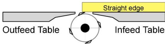
4. Fine tune table height to set depth of cut to zero. When properly set, cutters should be barely scraping the straight edge when cutterhead rotates.
