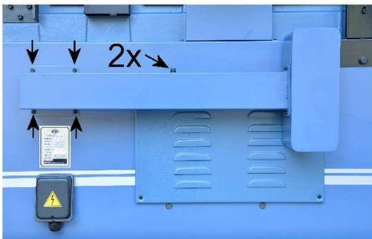
3. Raise the control panel to its operational position, then remount it back to the cabinet.
