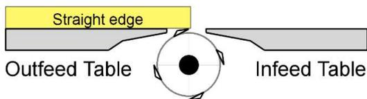
6. When outfeed table height is properly set, cutters should be barely scraping the straight edge when cutterhead rotates. Follow the next section to make adjustments as needed.
