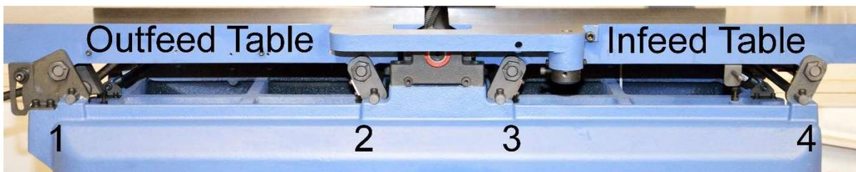
7. Locate and loosen the set screws for locking the eccentric nuts as shows in the pictures:
