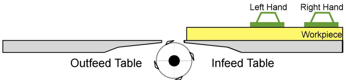
7. Feed a small section of stock across the cutterhead with pressure against the fence and the infeed table.
