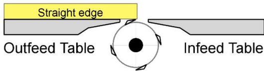
4. In each position, carefully rotate the cutterhead. When outfeed table is in parallel with cutterhead, cutters should be barely scraping the straight edge when cutterhead rotates.
