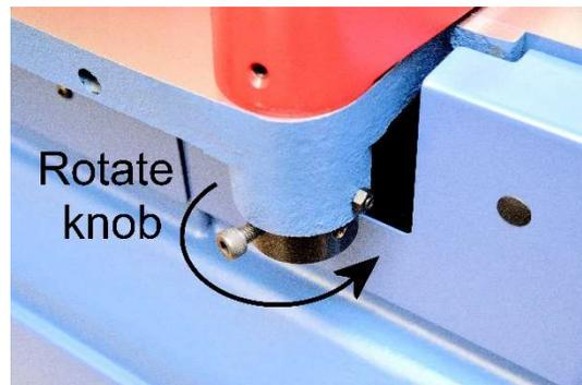
**NOTICE:** There are four screw holes on the knob. If the cap screw gets in the way while the knob rotates, relocate the screw and tighten when the knob is rotated to the proper position.
