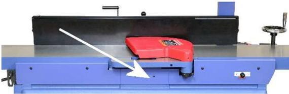
4. Remove all metal four metal panels that conceals the parallelogram mechanism.
