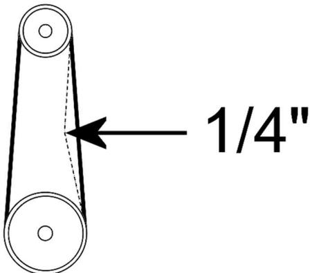
4. If V-belt tension needs to be adjusted, loosen both lower motor mounting bolts (#1). Lower the motor until proper belt tension is reached. Secure the motor mounting plate by tightening both upper mounting bolts (#2), and the lower mounting bolts.
