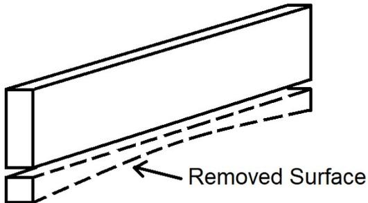
3. Set depth of the cut to the minimum amount to obtain a straight edge. Do not set cuts deeper than 1/8" in a single pass.
