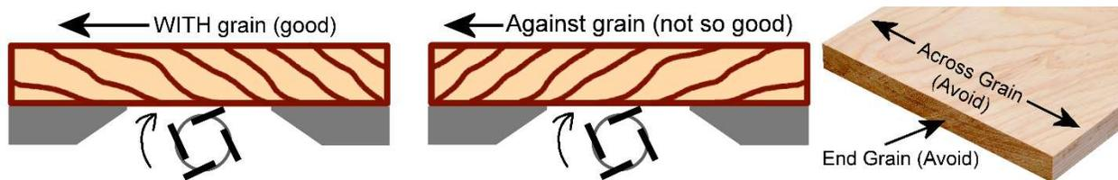
Sometimes it is impossible to cut with grain for the entire length of a workpiece. In this case, try feeding the workpiece in opposite direction and see what works best. Reducing the depth of cut and feed rate can also help improving cut quality.
