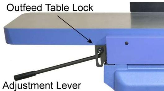
3. Adjust outfeed table height with the lever. With a straight edge sitting on the outfeed table, cutters should be barely touching the straight edge when cutterhead rotates.
