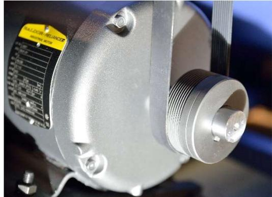
If the belt is too tight to remove, temporarily loosen the upper mounting bolts (#2). Raise the motor to loosen the belt, and remove it from the pulleys.
