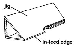
To perform a bevel-edge cut, the in-feed edge of the ig is placed against the infeed fence and clamped to the table as shown in Fig. 31. The outfeed fence is moved forward as necessary to compensate for the cut.
