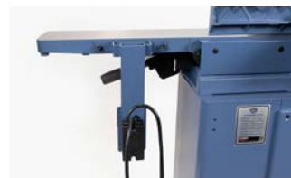
Easy assembly for power perch, simply rotate 180 degrees.
