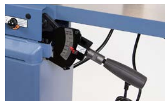
Infeed table adjustment and lock.
