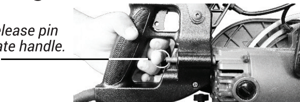
Figure 6. Handle releasing for rotation.
