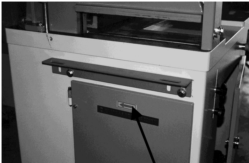
SAWBLADE RUNNING DIRECTION ARROW SIGN
