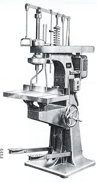
"Oliver" No. 73-T Single Spindle Borer with single speed motor and V-belt drive to spindle. Spindle speed: 3000 r.p.m.
