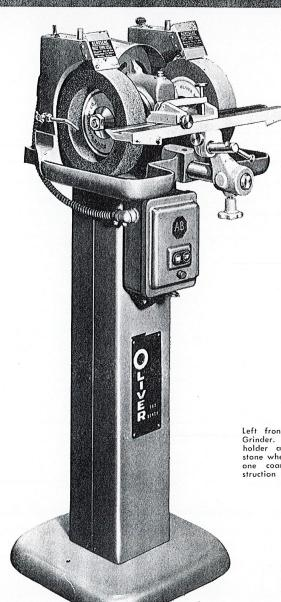
Left front view of No. 383 Grinder. Note adjustable tool holder as well as two oilstone wheels — one fine grain, one coarse grain. Its construction is rigid and sturdy.
