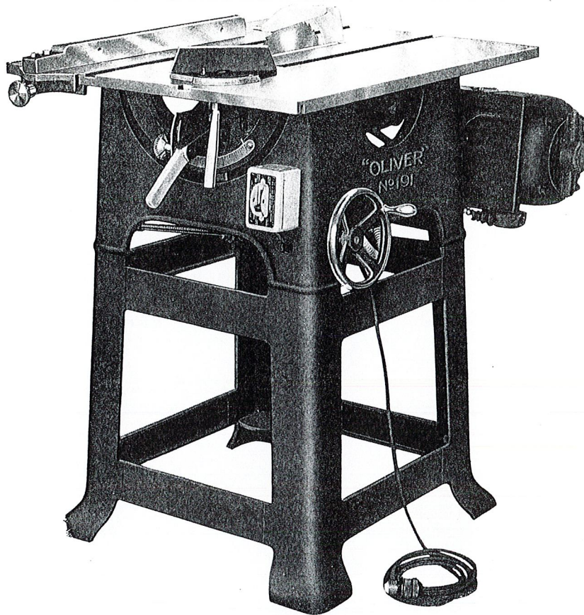
Front View from Right Side Showing Position of Motor and Saw in Normal Position and the Ripping Fence at the Left of Saw to Show its Use on Either Side.
