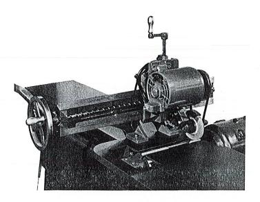
In the picture above, the bar is located accurately by the two tapped holes. The cutterhead or cylinder is located by the dowel pin. The motor bracket is clamped to the slide block by a hand knob, and the slide block is actuated by the crank shown at the left end. The cylinder remains stationary while the grinding wheel is fed taking a light cut. The next knife is brought in place by pulling out the dowel pin and rotating the cylinder by hand.
