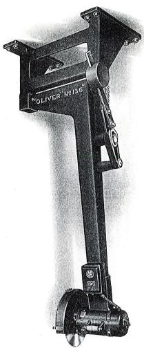
Enclosed Safety Switch can be locked in off position. Alemite system of lubrication used.
