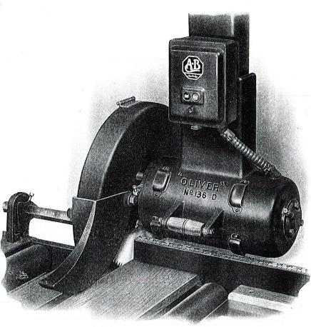
The Motor Arbor Head is made with light metal motor housing. The steel front guard is furnished as an extra. Note the semi-circular guard, hinged for changing saw.
